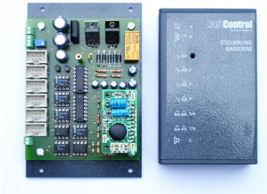
Figure 23 – Open control unit with sound module inserted (Version 2006)
