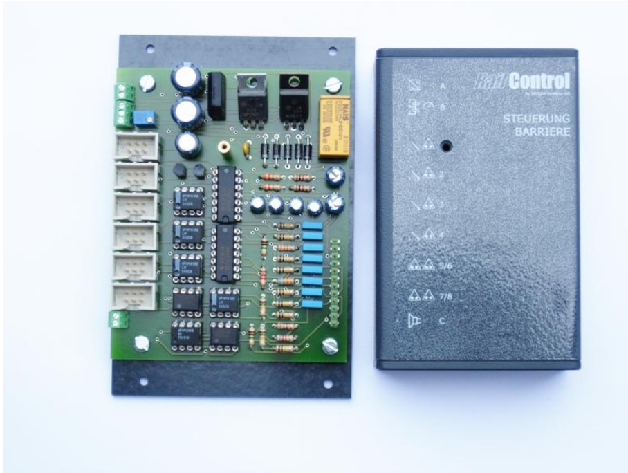
Figure 22 – Open control unit without sound module (Version 2006)
