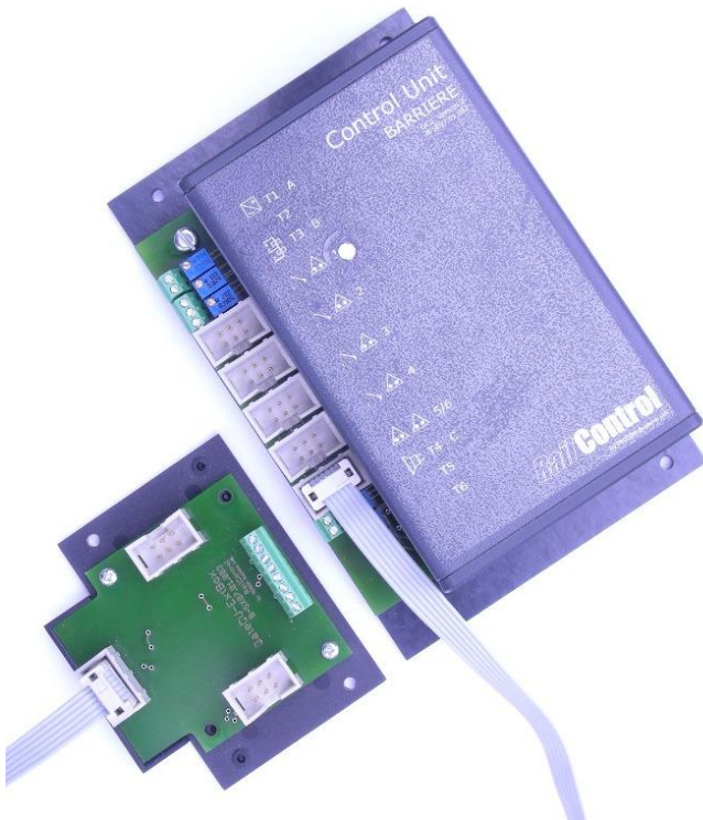
Figure 47 – Extender-Box connected to the Control Unit on connector 5/6
